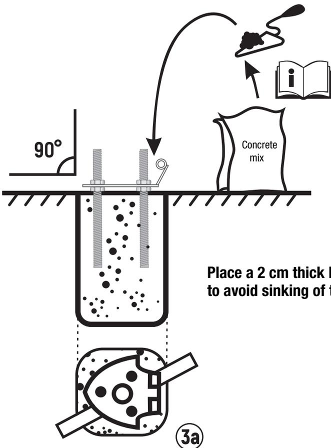
Place a 2 cm thick board under the hinge plate to avoid sinking of the ground attachment
