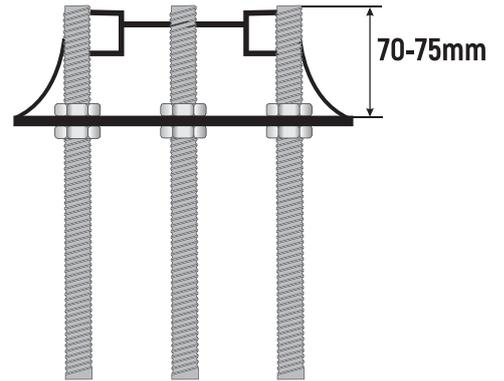
③ Fill the hole with concrete
